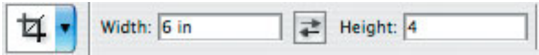
FIGURE 11.7 With the Crop tool selected, the Photoshop Control Bar lets you specify an aspect ratio for cropping.
